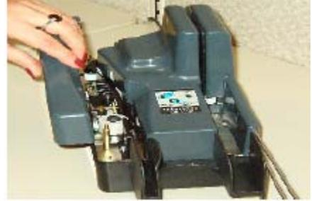
4. Unscrew the brass screw and gently open the scanner camera faceplates.
